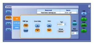
Select the source (Channel, Math, or Ref) and assign the Voltage and Current channels.
